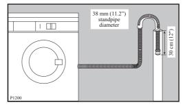
When discharging into a standpipe ensure that the top of the standpipe is no more than 90cm (35.4") and no less than 60cm (23.6") above floor level.
